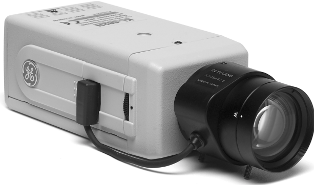
The KTC-840CE accepts both C- and CS-mount lenses.
